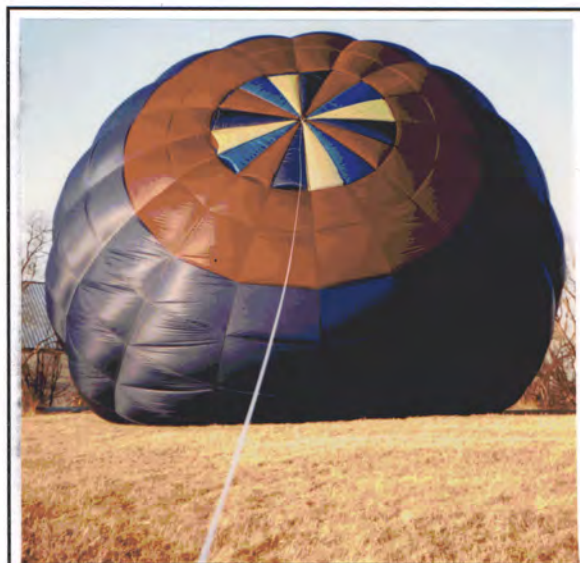
Looking at Ken Kennedy's 77,500 cubic foot envelope with an 18 foot parachute top. The envelope weight is 135 pounds. It was built from lightweight silicone coated fabric.
