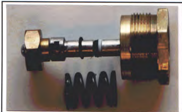
This is a Rego 7553T blast valve bonnet assembly. The little ring of rubber around the valve stem was sheared off as the bonnet was reinstalled in the valve body. The problem appears to be the result of lack of chamfer in the bonnet bore. Read the text for more details.
