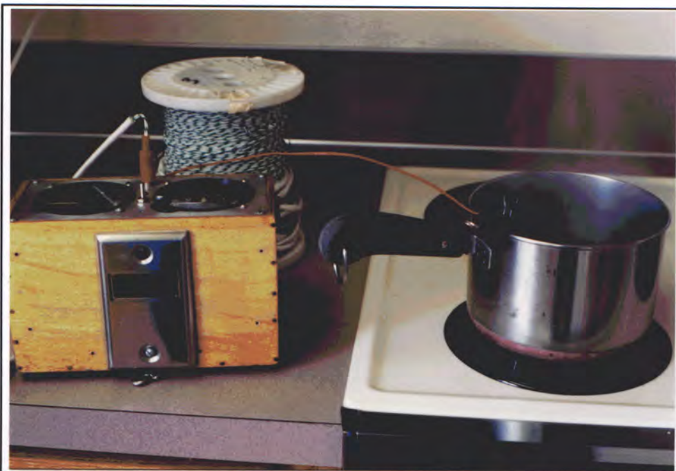
Figure 2: This photo shows the Castaway instrument box and temperature sensor test.
