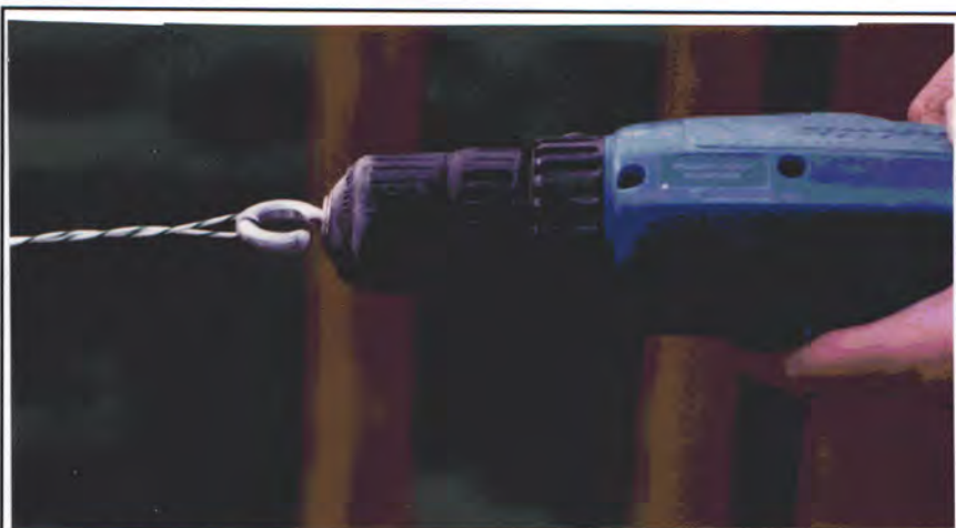
Figure 3: This photo shows the process for making a 'twisted pair' wire assembly. The length of wire is doubled in the middle at which point the bend is set in an eye-bolt in an electric drill. An assistant holds the loose wire ends and the wire is stretched horizontally about the ground. The drill is run until the wire is twisted every one to two inches.
