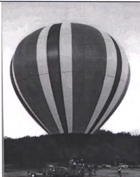
Figure 1: This set of photos, by Phil MacNutt, shows the change in envelope shape due to loading. In the top photo the balloon is loaded to a temperature of 110°F. In the bottom photo the envelope is loaded to maximum gross test load at 248°F.
