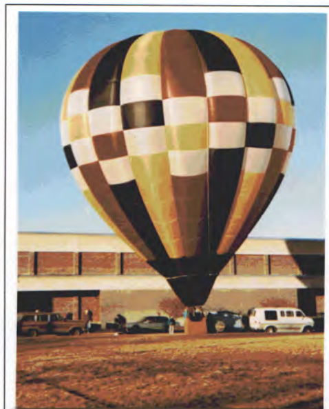
Ken Kennedy's new envelope built using light weight parachute type silicone coated fabric. The size is AX-7. It required 301 hours to build
