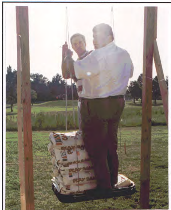
Figure 1. The Gross basket is hung by its vertical support cables. An asymmetric test load consisting of 450 pounds of sand has been loaded on one end of the basket.
