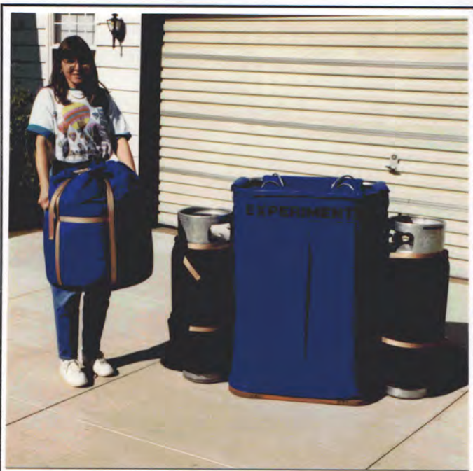
Figure 1. Kaye Knotts is holding Mike Emich's envelope, part of his very light balloon system. While Mike chose to obtain an 'experimental' airworthiness certificate for this balloon, it will qualify under FAR Part 103.
